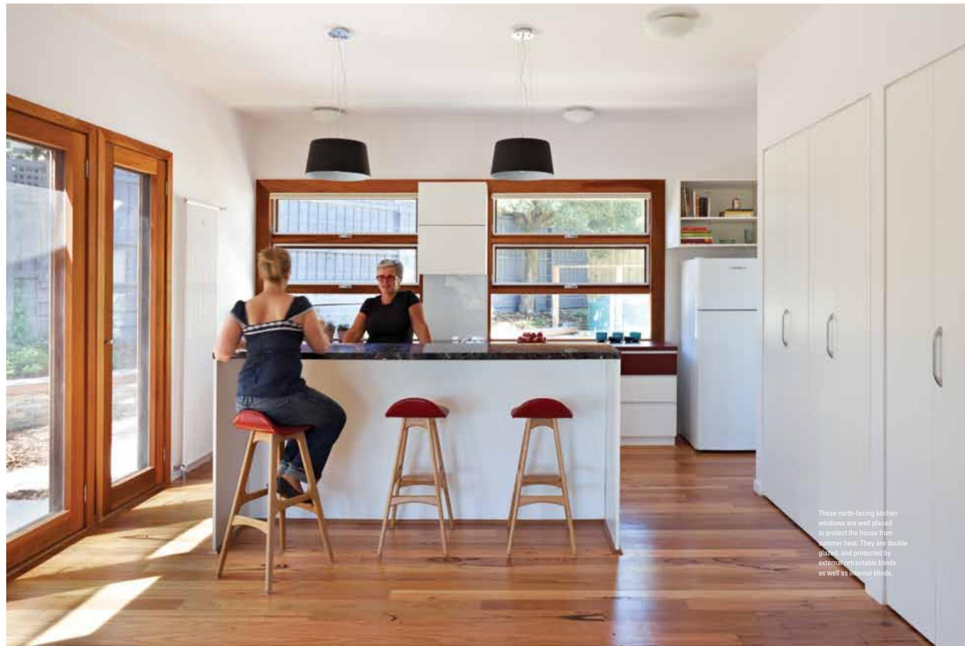
These north-facing kitchen windows are well placed to protect the house from summer heat. They are double glazed, and protected by external retractable blinds as well as internal blinds.
